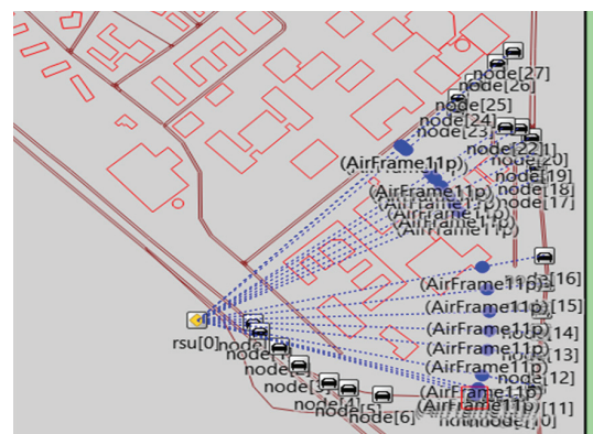
Figure 4. RSU sending alerts in the network using Airframe.
